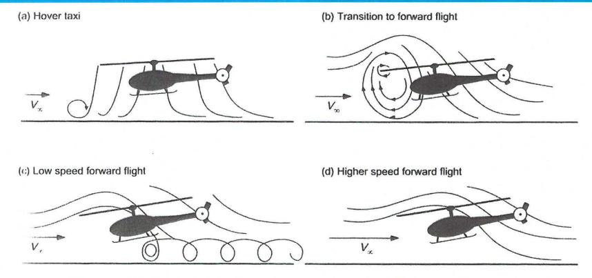
**Figure 5.37** Flow characteristics for a rotor in forward flight near the ground: (a) hover taxi. (b) transition to forward flight. (c) low speed forward flight. (d) higher speed forward flight. Adapted from Curtiss et al. (1984, 1987).
