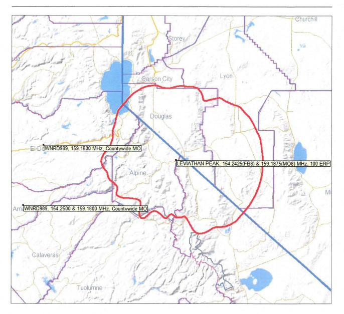
Proposed Frequency: 154.2425 MHz, FB8, Centralized trunked Relay 159.1875 MHz, MO8, Centralized trunked Mobile
